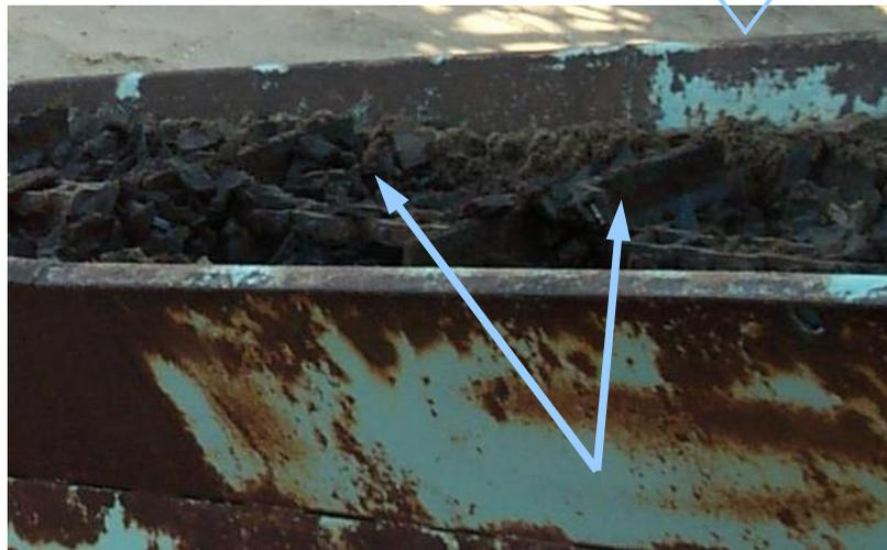
**Image 2: Enlarged Feeder mechanism image showing TDF and Hog fuel mix**
